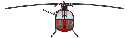
Figure 3-27. When a helicopter rotor is not turning, gravity causes the blades to droop. But when the rotor is turning, centrifugal force holds the blades straight out.
